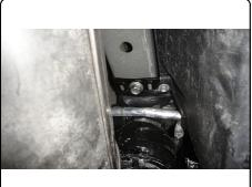
5. Raise the hitch over the exhaust and align the holes in the hitch with the weldnuts in the frame. Secure the hitch to the frame using the supplied M12-1.25 hex bolts and 1/2" conical toothed washers. Torque all 12mm hardware to 86 ft-lbs.
