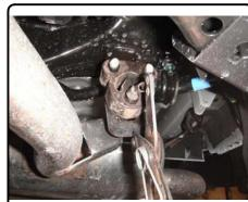
4) Raise hitch into position and secure with hex bolts and conical washers as shown in the diagram above.
