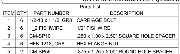
**REVERSE PULL FISHWIRE** TECHNIQUE ATTACH FISHWIRE TO CARRIAGE BOLT AND SLIDE SPACER ONTO FISHWIRE. PUSH THE BOLT THRU THE HOLE FOLLOWED BY THE SPACER (AS SHOWN). PULL BOLT BACK INTO POSITION, PROTRUDING FROM THE FRAME.
