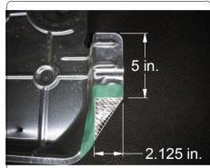
4. Enlarge the attachment holes along the bottom of each frame rail and the hole on the outside of each frame rail. Fishwire 1/2" carriage bolts and SP10 spacers through the access hole to the forwardmost hole and the outside holes on each frame rail.
