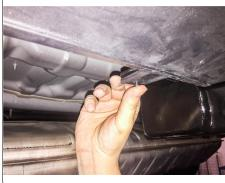
9. Torque all 1/4" hardware to 10 ft-lbs and all M10 hardware to 45 ft-lbs. Reinstall following steps 2 - 4 in reverse order.
