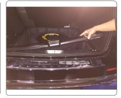
5. Inside trunk locate and remove bumper beam nuts, (2) on each side, using 16mm socket.
