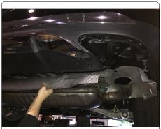
4. Remove trunk liner guard using T-30 socket to remove screw. Gently unclip trunk liner guard and remove trunk contents to expose bumper beam nut inside vehicle. Set aside trunk contents and trunk liner guard for reinstallation.
