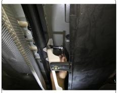
2. Lower exhaust by removing rubber isolator from hanger attached to vehicle frame, (1) on each side. Support exhaust to prevent damage.
