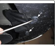
2. Reverse fishwire (2) 7/16-14 x 1 1/2" carriage bolts and CM-SP2 spacers into the existing hole in the bottom of the frame rails leaving the fishwires attached.
