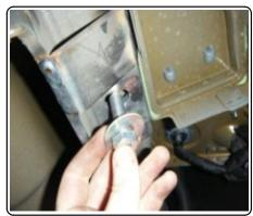
6.Torque M12 hardware to 79 lb-ft and 1/2" hardware to 110 lb-ft. Raise exhaust back into position.
