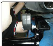
4. Reverse fishwire 1/2" carriage bolt and CM-SP10 spacer through existing hole in passenger side frame rail.
