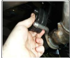
2.Remove (2) rubber isolators from muffler. Remove exhaust hanger and/or exhaust hanger with existing tow loop. Return hangers and hardware to vehicle owner.
