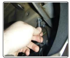
5.Raise hitch into position and secure with supplied M12 hex bolts and 1/2" conical toothed washers into existing vehicle weldnuts. Secure 1/2" carriage bolt with supplied hex flange nut.
