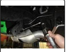
3. Remove the (2) existing hex bolts from the frame on both sides of the vehicle.
