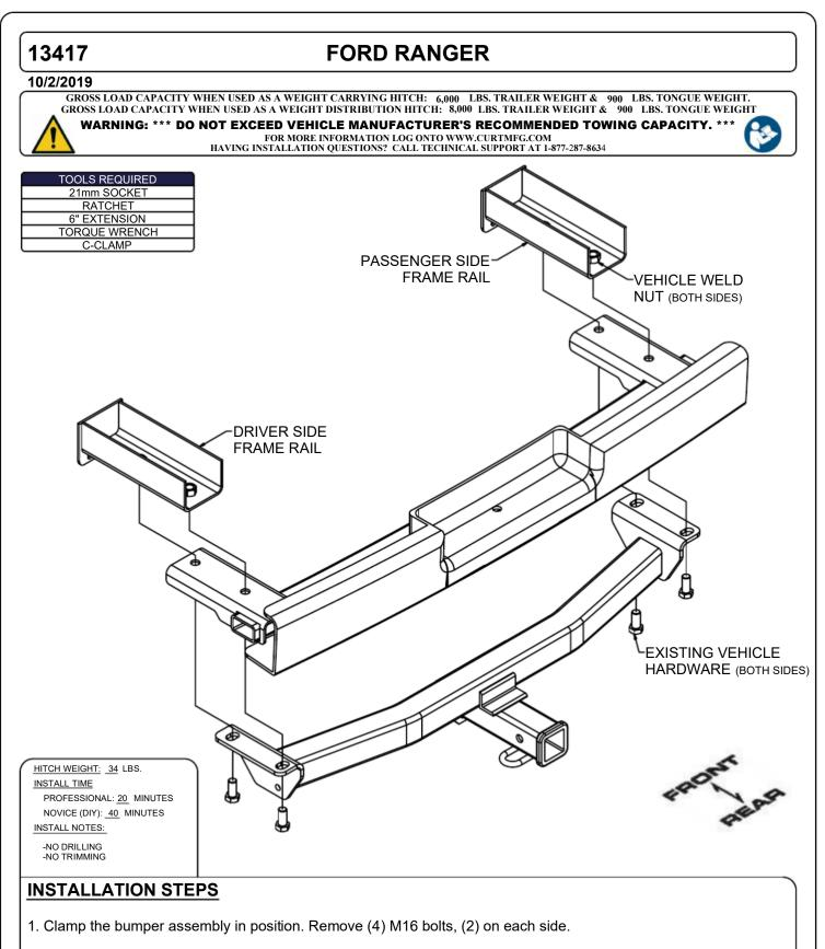
2. Raise hitch into position, use existing hardware removed in step 1 to secure hitch and assembly to vehicle.
