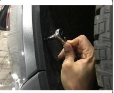
2. Remove (4) M10 nuts with a 15mm socket from the top bumper attachments, set nuts aside for re-attachment, (2) each side. Remove (4) M10 bolts with a 15mm socket from the bottom bumper attachments, (2) each side. Return the bumper beam and bolts to the vehicle owner.
