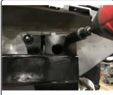
4. Tighten all 1/2" fasteners with torque wrench to 110lb-ft and all M10 fasteners to 45lb-ft.
