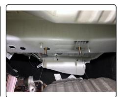
8. Raise hitch into position. (**NOTE**: Hitch will be positioned between the upper and lower kick sensor wires if equipped as shown in step 9.) Torque 1/2" hardware to 75 ft-lbs and torque M16 hardware to 146 ft-lbs.
