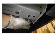
5. If kick sensor is present, remove (4) of the (6) rivets using a drill along rear fascia, starting from driver side, to avoid damaging kick sensor while trimming. Replacement rivets are included.
