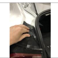
2. To remove tailight locate and remove (2) nuts, on each side, using 8mm socket. Unplug electrical harness and gently remove tailight. Set aside tailight for reinstallation. Remove exposed fascia screw using 10mm socket, on each side.
