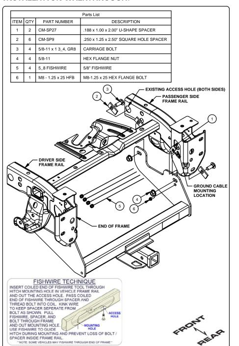
If present, remove the grounding cable from the rear of the passenger side frame rail.
