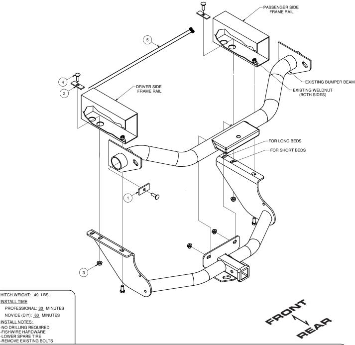
NOVICE (DIY): 60 MINUTES INSTALL NOTES: -NO DRILLING REQUIRED -FISHWIRE HARDWARE -LOWER SPARE TIRE
