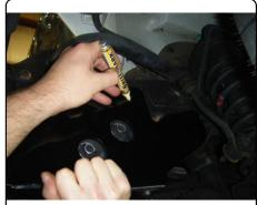
2. Lower hitch and drill (2) holes using a 9/16" drill bit.
