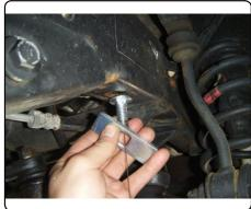
5. Thread fishwires through hitch mounting holes and raise hitch into position. Secure to frame using 1/2" flange nuts.
