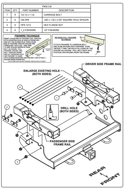
1. Raise hitch into position and mark (2) drill hole locations, as shown. **NOTE:** Lift driver side first so the bolt heads on the side of the frame go through the large holes in the hitch side plate and then raise hitch into position.
