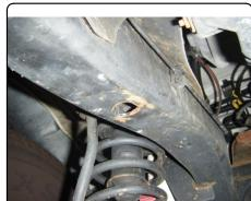
4. Fishwire (2) carriage bolts and (2) SP-6 spacers into position in the side of each frame rail. Reverse fishwire (1) carriage bolt and (1) SP-6 spacer into position in the bottom of each frame rail. NOTE: Leave fishwires attached to all hardware to prevent loosing in frame.
