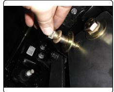
7. Reposition and level bumper by pushing up on it while tightening the hardware. Torque 5/8" hardware to 150 ft-lbs and M12 hardware to 86 ft-lbs.
