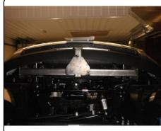
6. Insert spacer plate (6) between the frame and hitch side plate. Insert two 5/8" x 4" hex bolts (1) with a lock washer (2) and washer (3) on each. Insert in through the side plate / spacer and out the frame, as shown on page 2. Attach using two 5/8" hex flange nuts (4), two spacers (6) and repeat on the other side.
