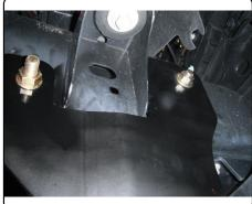
5. Torque all 1/2" fasteners to 110 lb-ft and all 5/8" fasteners to 210 lb-ft.
