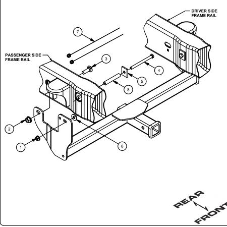
1. Remove the lower air dam on 2011 and newer trucks by removing (2) nuts with a 15MM socket. Trim the lower plastic bumper fascia as required using the diagram below as a reference only.
