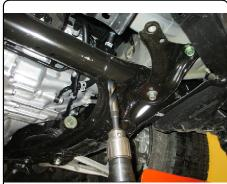
4. Raise hitch into position. Loosely install M12 x 40mm bolt with a conical toothed washer with (2) CM-SP50 spacers placed on top of each side plate and in between vehicle bracket and side plate.
