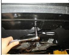
2. Remove (2) plastic push pins from crossmember, (1) on each side. Using a phillips screwdriver, remove (2) screws from vehicle panel, (1) on each side. Remove panel and return to owner.
