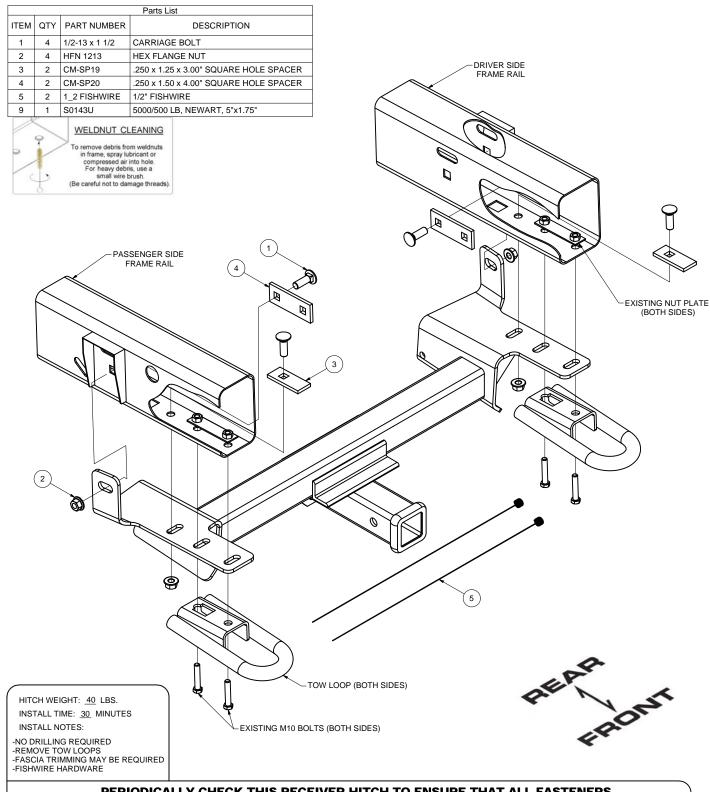
PERIODICALLY CHECK THIS RECEIVER HITCH TO ENSURE THAT ALL FASTENERS ARE TIGHT AND THAT ALL STRUCTURAL COMPONENTS ARE SOUND.
