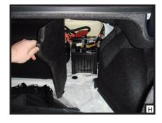
5. Route the black wire behind the felt trunk liner to the battery. The battery is located on the passenger side behind the back seat in the trunk. [H] Using a 10 mm socket remove nut on on both battery terminals. Remove the negative (-) battery cable. Connect the black power wire terminal ring to the positive (+) battery terminal. Reconnect the negative (-) battery wire. Insert the 10 AMP fuse into the inline fuse holder.
