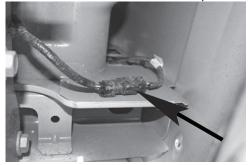
Figure 1 3. Starting on driver's side position RV harness connectors ends containing Yellow wires between separated vehicle harness connectors shown in Figure 2. Press connectors firmly into vehicle connectors until they lock into place and slide Red lock on factory connector. Pull on connectors to ensure locks are engaged.
