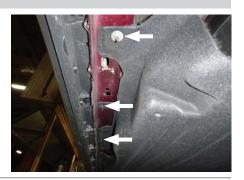
Route the 4-flat over to the rear of the driver-side front wheel well. Use fish wire to route from the top and down in between the inner and outer fender. Pull the 4-flat up to the engine compartment
