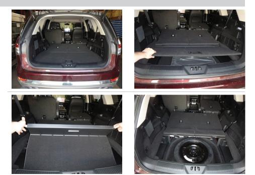
Using a panel trim removal tool, release the push fasteners securing the skid plate in place. Separate the hatch sensor connector taking care not to damage the locking tabs. Set the skid plate aside.
