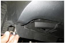
Starting on the outer edges, pull the fascia panel out while using a non-marring pry tool to release the four clips from each fender.
