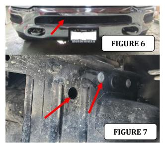
**Step-7** Locate the existing hole and the existing bolt on the bumper beam. Figure 7. Remove the factory bolt. NOTE: Use a hammer to push out the factory carriage bolt.
