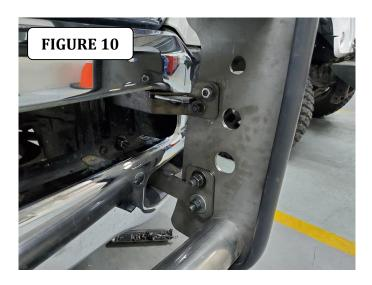
**Step-10** Place the Grille Guard over the lower and upper brackets. Figure 9. Secure the lower brackets using (2)  $1/2 \times 1 \cdot 1/2$ " hex bolts, (4) 1/2" flat washers, (2) 1/2" lock washers and (2) 1/2" hex nuts. Secure to upper brackets using (2)  $3/8 \times 1 \cdot 1/4$ " hex bolt, (2) 3/8" flat washer, (2) 3/8" lock washer and (2) 3/8" hex nut. Leave loose. Figure 10.
