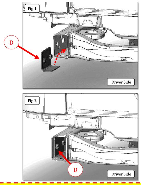
**Note:** It is recommended to apply a strip of duct tape to hold the nut plate in place inside the frame rail prior to positioning the Rockline rear bumper on the frame rails and installing the bolts.
