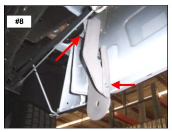
**STEP-9** ATTACH THE DRIVER SIDE STEP TO THE FRONT AND REAR BRACKETS USING (1) 1/2" X 2" HEX BOLT, (1) 1/2" FLAT WASHER AND (1) 1/2" LOCK WASHER FOR EACH BRACKET.
