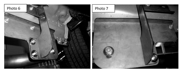
**6.** Attach the side bar to the center bracket using (1) 5/16" x 1" hex bolt Black P., (1) 5/16" flat washer Black P. and (1) 5/16" spring lock washer Black P. Leave the nuts loose for final adjustment. **(Photo 8)**
