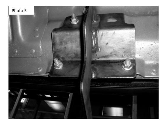
5. Attach the side bar to the front and rear bracket using (2) 1/2" x 2" hex bolts, (2) 1/2" flat washers and (2) 1/2" spring lock washers. Leave the nuts loose for final adjustment. (Photo 6 & 7)
