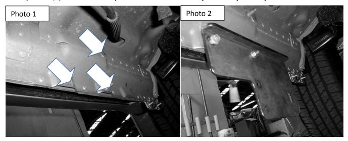
2. Install the auxiliary bracket using (1) b M8 hex nut Gray P., (1) 5/16" flat washer Gray P. and (1) 5/16" spring lock washer Gray P. Then attach the auxiliary bracket to the front bracket using (2) 5/16" carriage head bolt Black P., (2) 5/16" flat washers Black P., (2) 5/16"spring lock washers Black P. and (2) 5/16" hex nuts Black P. Leave loose for final adjustment. (Photo 3)
