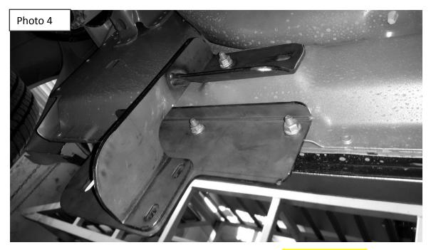
**4.** Locate the M8 welded bolts in the rocker panel at the middle of the cab and install the center bracket using (3) 5/16" flat washers Gray P., (3) 5/16" spring lock washers Gray P. and (3) M8 hex nut Gray P. Leave the nuts loose for final adjustment. **(Photo 5)**
