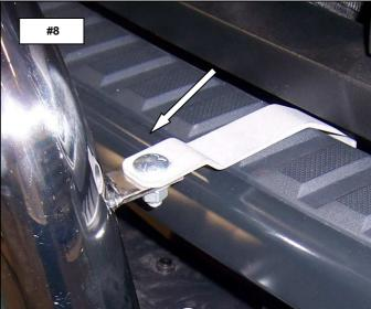
**Step-8** Align the Rhino Charge bar and bracket assembly and tighten all nuts and bolts. Remember to check and re-tighten the hardware periodically.
