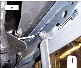
**Step-4** Position one of the upper brackets behind the bumper, so the longer leg of the bracket extends out between the top of the bumper and the bottom of the grille. **Photo #5**
