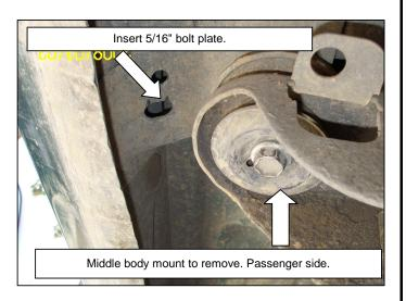
**5.** Install the middle bracket and attach with bolts before removed. Locates the hole that is in the rocker of the vehicle and inserts 5/16" bolt plate.
