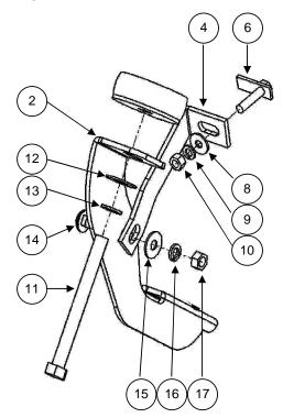
Use ratchet & 18mm - 19mm - 9/16" - 1/2" hex socket. Remove the bolt OEM with: ratchet & 18mm hex socket.
