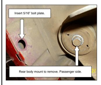
7. Install the middle bracket and attach with bolts before removed. Locates to the rubber plug that is in the rocker of the vehicle, remove and insert 5/16" bolt plate.
