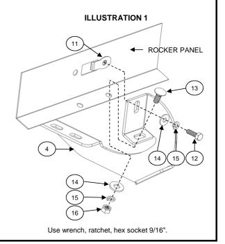
**NOTA:** Models 2009 - 2010 insert 3/8" bolt plate, gasket vinyl, middle part, attach with: 1 3/8" flat and lock washers, 3/8" hex nut. In lower part attach with: 3/8 x 1" carriage head bolt, 3/8" flat and lock washers, 3/8" hex nut. **SEE PICTURE 3 & ILLUSTRATION 2.** Leave loose. Repeat in opposite side.
