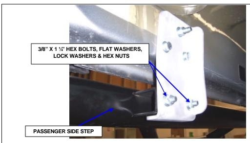
**STEP 5.** ATTACH THE PASSENGER SIDE STEP TO THE MOUNTING BRACKETS USING (2) 3/8" X 1 1/4" HEX BOLTS, (4) FLAT WASHERS, (2) LOCK WASHERS AND (2) HEX NUTS FOR EACH BRACKET.
