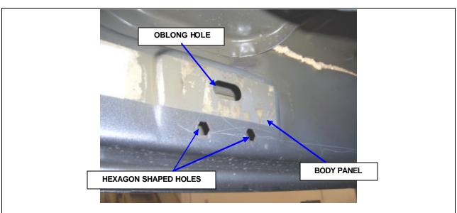
**STEP 1.** THIS INSTALLATION USES (3) MOUNTING BRACKETS PER SIDE. BEGIN BY INSTALLING THE PASSENGER SIDE FRONT BRACKET. LOCATE THE (2) HEXAGON SHAPED HOLES IN THE UNDERSIDE OF THE BODY PANEL AT THE FRONT OF THE CAB AND REMOVE THE TAPE COVERING THE OBLONG HOLE.
