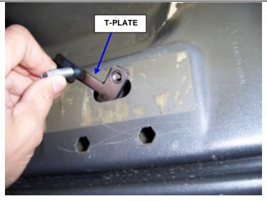
**STEP 2.** INSERT (1) OF THE T-PLATES THROUGH THE OBLONG HOLE IN THE BODY PANEL AND POSITION THE PLATE INSIDE THE PANEL AS SHOWN. PLACE (1) OF VINYL GASKETS TO THE T-PLATE.
