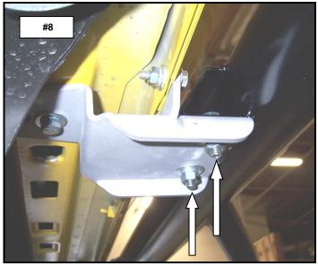
**STEP 7.** ALIGN THE SIDE STEP WITH THE VEHICLE AND TIGHTEN ALL MOUNTING BRACKET AND SIDE STEP NUTS AND BOLTS.
