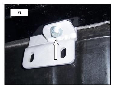
Step-5 Passenger side Center bracket installation.
