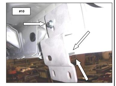
Step-6 Passenger side rear bracket installation.
