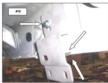
Step-6 Passenger side rear bracket installation.
