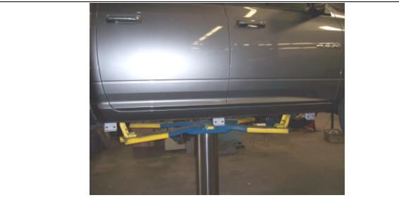
STEP 4. REPEAT THE ABOVE PROCEDURE TO INSTALL THE CENTER AND REAR MOUNTING BRACKETS.
