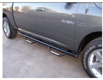
**STEP 6.** ALIGN THE SIDE STEP WITH THE VEHICLE AND TIGHTEN ALL MOUNTING BRACKET AND SIDE STEP NUTS AND BOLTS. REPEAT THE ABOVE PROCEDURE TO INSTALL THE DRIVER SIDE BRACKETS AND SIDE STEP.
