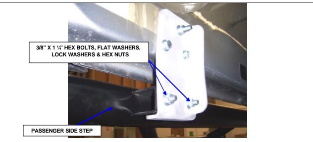
**STEP 5.** ATTACH THE PASSENGER SIDE STEP TO THE MOUNTING BRACKETS USING (2) 3/8" X 1  $\frac{1}{4}$ " HE X BOLTS, (4) FLAT WASHERS, (2) LOCK WASHERS AND (2) HEX NUTS FOR EACH BRACKET.
