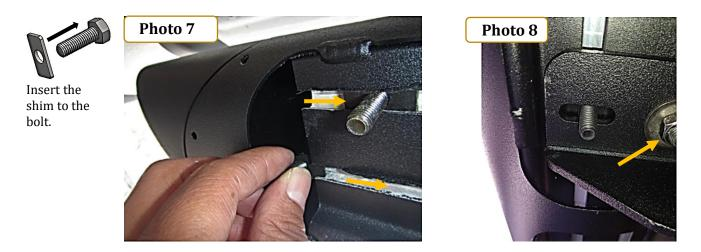
**Step-9** Align the side step with the vehicle and tighten all brackets and side steps nuts and bolts. Repeat the above steps to install the passenger side brackets and side step. Remember to check and retighten the nuts and bolts every six months.
