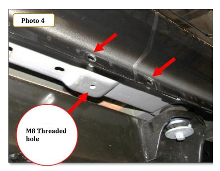
**Step-4** Attach one of the driver side Front/Center brackets to the pinch mold using (2)  $\frac{1}{4} \times 1^{n}$  hex. Head bolt, (4) 1/4" Flat washer, (2) 1/4" Lock washer and (2)  $\frac{1}{4}$ " hex nut, and to the underside of the body using (1) Sems M8x30 Hex bolt. **Photo 5 & 6.** Leave the nuts and bolts loose for final adjustment.
