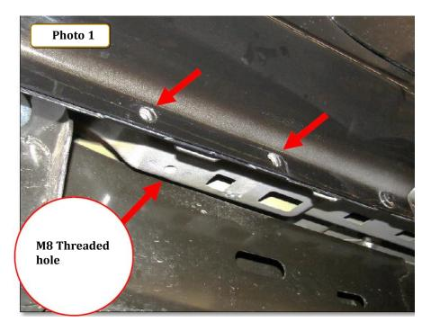
**Step-2** Attach one of the driver side Front/Center brackets to the pinch mold using (2)  $\frac{1}{4} \times 1^{n}$  hex. Head bolt, (4) 1/4" Flat washer, (2) 1/4" Lock washer and (2)  $\frac{1}{4}$ " hex nut, and to the underside of the body using (1) Sems M8x30 Hex bolt. **Photo 2 & 3.** Leave the nuts and bolts loose for final adjustment.
