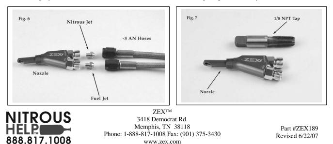
nozzle in a metal duct. Just drill a 11/32 inch hole where you want to mount the nozzle, tap the hole and install the nozzle. Once the nozzle is installed, place the appropriate tuning jets in the nozzle and attach the 2-foot long, -3AN hoses to the nozzle jet fittings and the nitrous management unit (Fig.6).
