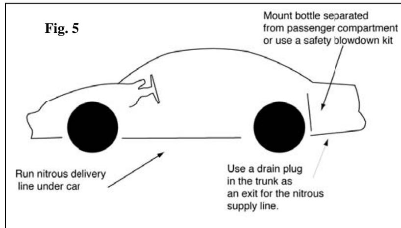
**3. Mount nitrous delivery line under the car** - When routing the nitrous delivery line under the car, try to use the subframe as a conduit (Fig. 5). This protects the line and eliminates the need to use clamps. The supplied cable ties work if you can run the line higher in the under-body so that it's safe from the road level obstacles such as speed bumps. For the pro-race look, you can use steel loom clamps with rubber sheathing to fasten the line to the body.
