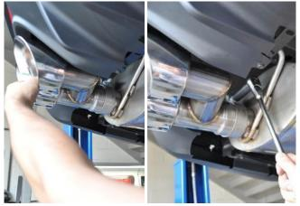
1. CAREFULLY insert the tip assembly into the driver side muffler outlet pipe and snug the clamp using a 15mm socket, 3/8" driver ratchet and 3" extension.
