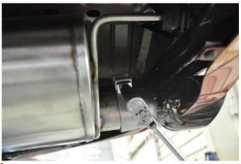
1. Loosen the two clamp bolts at the inlet of the current CORSA driver and passenger tip assemblies using a 15mm socket and a 3/8" ratchet, and a short extension.
