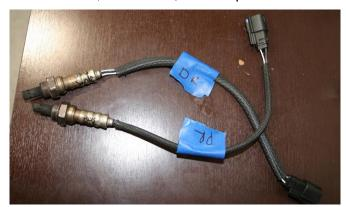
3. Remove the rear O2 sensors and label their positions using a 22mm wrench or O2 sensor socket and 3/8" ratchet. PRO TIP: Label on the connector or the sensor body itself. EXAMPLE: DR for Driver Rear. PR for Passenger Rear.
