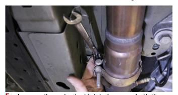
Loosen the spherical joint clamp on both the catalytic converters using a 13mm wrench.
