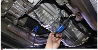
**9.** Plug O2 sensors into off road pipes as shown in picture.
