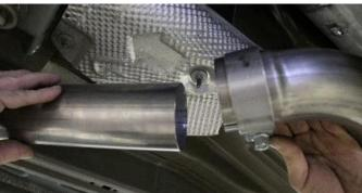
12. Add a 2.75" clamp to each of the CORSA X-Pipe inlets. Insert the CORSA Inlet Elbow Pipes into the X-Pipe inlets. Snug connection using a 15mm socket or wrench.
