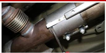
**1.** On the driver side, use a flat screwdriver to pry the clamp spring clip from the retainer pin on the H-Pipe repeat on passenger side.
