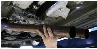
9. Pull the front of the H-Pipe from the spherical clamp joint on both sides and side the outlet ends from the sleeve clamps to remove the Hpipe assembly from the vehicle. NOTE: The clamps on the outlet end are reused, so if they stick to the H-Pipe assembly, remove them and re-install onto the axle pipes.
