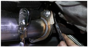
**4.** Tighten with a 15mm socket or wrench, secure the off road pipe with the supplied nuts.
