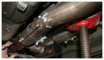
4. Support the factory axle pipes and the driver catalytic converter with a jack stand or similar device. DO NOT let the exhaust droop as it may damage the rear bumper cutouts
