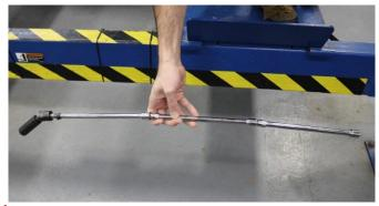
Locate the flange connecting the passenger catalytic convertor to the manifold, from the top of vehicle in the engine bay remove the top nut nearest to the firewall using three 12" long 3/8" extensions, 3/8" swivel, and deep 15mm socket.
