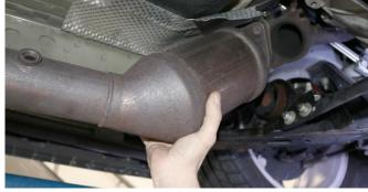
Remove the driver/passenger catalytic converter pipes from the vehicle.
