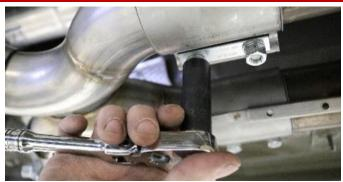
11. Install the outlet of the CORSA X-Pipe assembly into the factory sleeve clamps at the inlet of the axle pipes. Using a 15MM socket or wrench to snug the 2 bolts on the sleeve clamp Repeat for opposite side.
