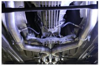
14. Insert the inlet elbow pipes into the off-road pipe outlet as shown, secure the inlet elbow connection using a 15mm socket or wrench.
