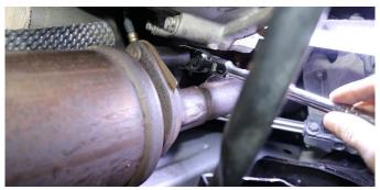
10. Locate the flange connecting the driver catalytic convertor to the manifold. Use a 15mm socket and 3/8" ratchet to remove the two nuts. Repeat on passenger side, for the remaining nut. WARNING: The front section of the exhaust could drop down. Support it using a jack stand, screw jack, or similar device
