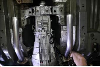
**6.** Make sure both driver/passenger off road pipes are aligned correctly before tightening down.
