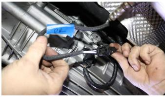
WARNING: Make sure you put the O2 sensors in the correct cat pipes as you marked them in the removal process.
