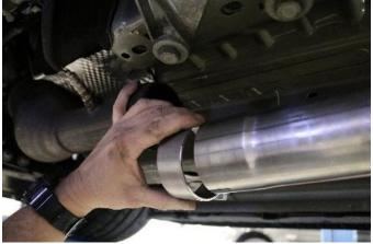
**13.** Adding a 2.75" clamp to the inlet side of each CORSA Inlet Elbow Pipe.
