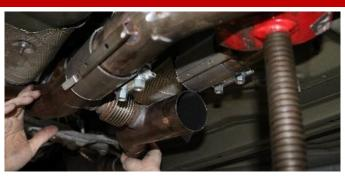
**8.** Slide both sleeve clamps towards the rear of the vehicle to free the end of the H-Pipe.
