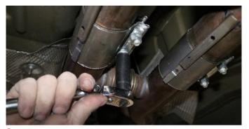
**6.** Using a 15MM socket or wrench, loosen the factory sleeve clamps (4 Bolts) after the H-Pipe assembly.
