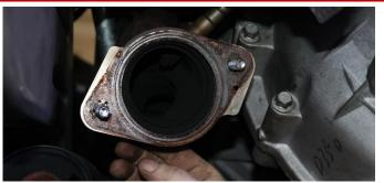
Locate the mounting hardware and the two gaskets from Removal Step 12. On the driver side, insert the two supplied bolts through the stock manifold flange from the top. Insert the gasket onto the bolts as show.
