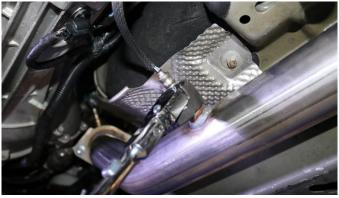
**8.** Install both driver and passenger oxygen sensors onto the off road pipes as shown, tighten with a 22mm O2 sensor socket or wrench.
