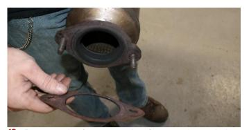
Remove the factory gasket from each catalytic converter. Save for Install Step 2 This concludes the factory exhaust removal. Part #: 14421
