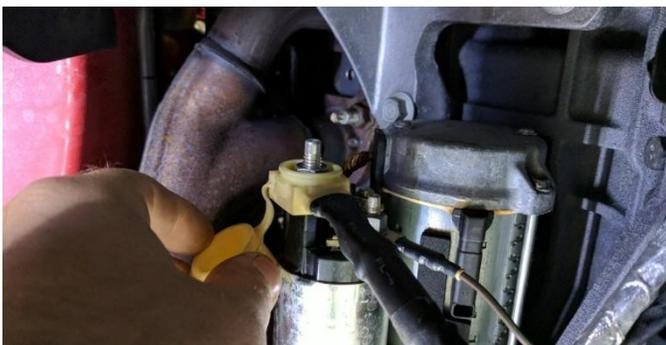
12. Reinstall the starter, secure it with the three 10mm bolts from **Removal Step 15** using a 1/4 drive ratchet and 10mm socket with 3" extension. Connect the starter wires using the ratchet with the 10mm and 13mm nuts.
