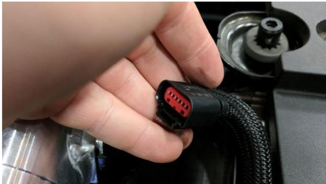
3. On the driver side, locate the harness connector for the mass air flow sensor. Release the red security clip by pulling the red clip toward the wires and then disconnect the wires from the sensor.
