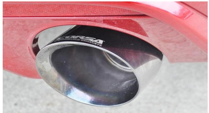
**22. The help of a second person is required for this step.** Ensure the exhaust tips are properly centered within the rear bumper valence. Tighten all clamps to 45ft-lb. Tighten the spherical flange nuts and bolts to 15ft-lb or 180in-lb using a 1/2" socket, extensions (as necessary), a torque wrench, and 1/2" box wrench.
