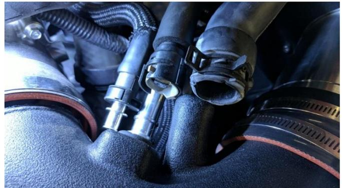
4. Disconnect the breather hoses in the bend of the intake duct using pliers to loosen the hose spring clamps. The third hose has a button-style clamp. Press the release buttons and carefully pull the hose off the barb. Aftermarket intake shown in picture for reference only.
