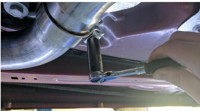
**21.** Begin the final alignment process by snugging all clamp bolts using a ratchet and 15mm socket. Align the adapter pipes so they are roughly parallel to the ground and running straight toward the rear of the vehicle. The pipe overlap between the elbows and at the inlet side of the X-Pipe should be slightly more than 1.5". With the system snugged, adjust pipe overlaps and check all clearances to heat shields, wiring harnesses, and chassis components.
