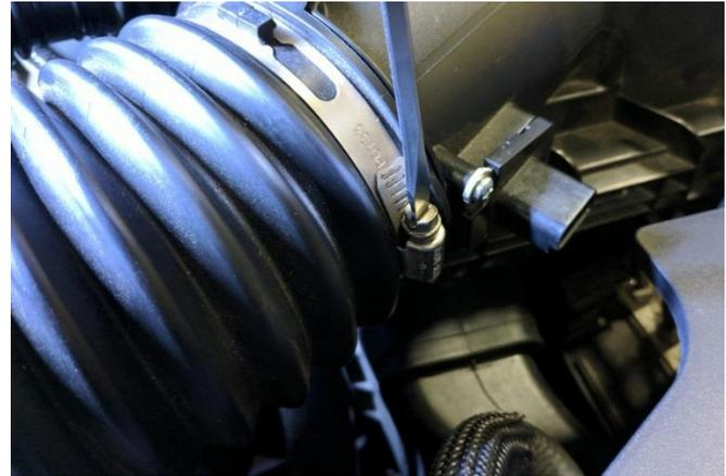
**25.** In the engine bay, reinstall the air intake box and secure it with the bolt from **Removal Step 5**. Tighten the hose clamp with a flathead screw driver or nut driver. Connect the airflow sensor cable and lock in place with the red tab. Connect the breather hoses to the intake duct.
