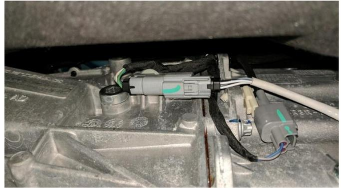
**20.** Repeat **Install Steps 15-18** on the driver side of the vehicle. **Driver Side:** Remove the harness connector from the transmission and rotate it down so the connector is on the bottom side of the mounting point with the open end facing the rear of the car. Connect the driver side rear O2 sensor.
