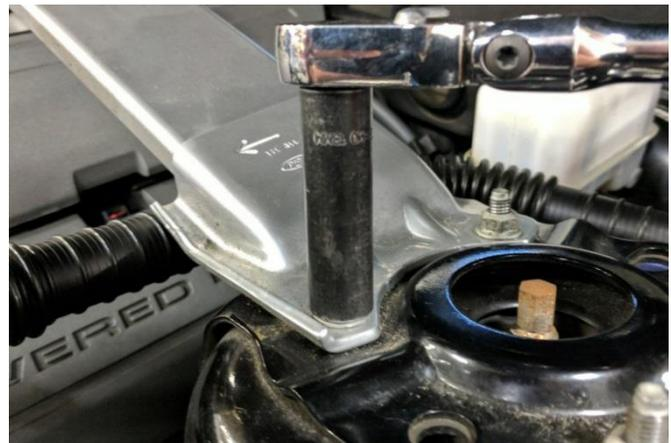
2. Remove the strut tower bar, if present, using a 15mm socket and 3/8" ratchet. **Save for reinstallation (Install Step 26).**
