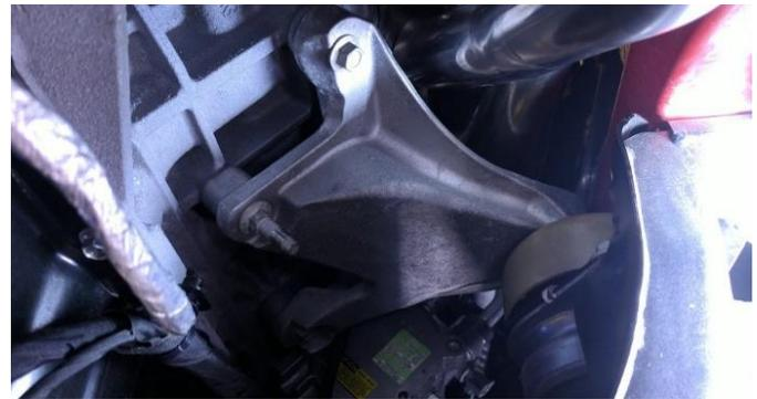
11. Reinstall the factory engine mount brackets using a ratchet and 13mm socket. **Passenger Side:** Ensure the top bolt in the front has a threaded stud on the hex end. Reinstall the ground strap and secure with the 15mm nut removed during **Removal Step 17**. Lower the engine back onto the engine mounts.
