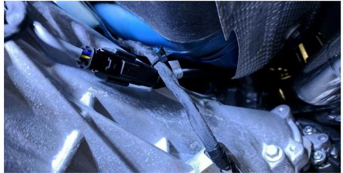
2. **'15-'17 & '18 Auto:** Install the passenger front O2 sensor extension wire. **PRO TIP:** Route it around the bellhousing at the rear of the engine. This keeps it tucked away from the header once installed. **'18 Manual:** Skip to **Install Step 3** - No extension is needed.
