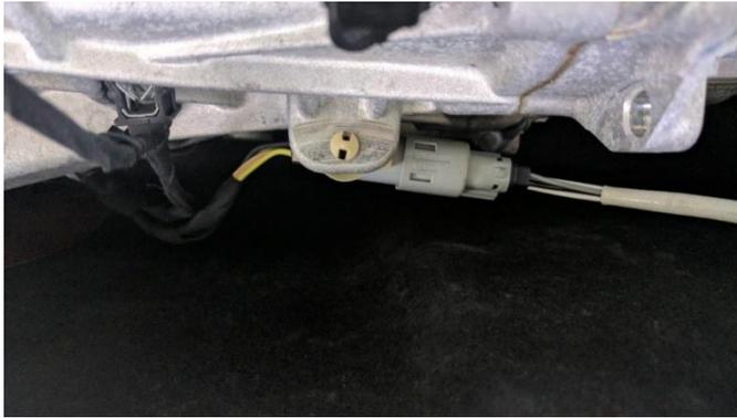
**19.** Connect the passenger side rear O2 sensor to the vehicle harness. (Located on the side of the transmission housing).
