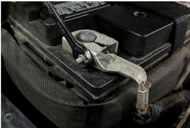
1. Remove the black negative battery cable using an 8mm wrench.
