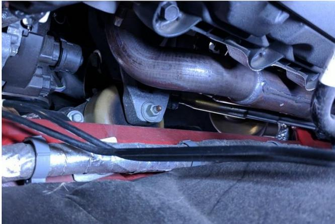
**24.** Secure the top of the engine mounts with the nuts removed during **Removal Step 6**, using extensions, a ratchet, and a 15mm socket.
