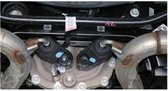
**4.** Use a 3/8" drive ratchet and 13mm socket to remove the bolt holding the driver side hanger grommet assembly. Save bolt for **Install Step 6**. Push up slightly on the exhaust and slide the hanger grommet assembly rearward to free it from the rear suspension sub-frame. Rotate the hanger grommet assembly a minimum of 90° so it will not interfere with the rear suspension sub-frame. Repeat for passenger side.
