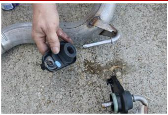
9. Remove the driver and passenger side hanger grommet assemblies from the axle pipe hangers using grommet pullers or a similar device. Save for Install Step 4.
