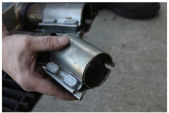
**8.** Remove both sleeve clamps from the stock cat-back and save for **Install Step 1**.
