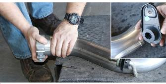
Install the passenger hanger grommet assembly from Removal Step 9 onto the front hanger of the CORSA passenger muffler assembly in the same position as it was installed on the stock exhaust. Install one 3" clamp on the muffler inlet pipe with the nut towards the ground, the bolt vertical and towards the inside of the vehicle.
