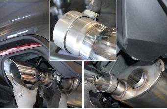
Install one 3" clamp on passenger non-valve tip assembly inlet pipe with nut towards the inside of the vehicle, bolt horizontal and towards the top. Slide tip assembly over muffler outlet pipe and tighten clamp using a ratchet and 15mm deep socket until tip assembly is snug on muffler outlet pipe. Repeat on driver side.
