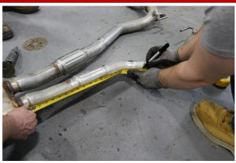
**13.** On the driver side, measure 19 3/4" away from the flange on the stock resonator, following the outside profile of the exhaust pipe.
