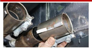
Slide the two sleeve clamps from Removal Step 8 over the stock exhaust pipes. If needed, bend back the locking tab to its original position. Confirm the button on the stock exhaust pipes is positioned correctly within the slots in the sleeve clamps, and the locking spring tab on the clamps is pushed on far enough to engage the button.
