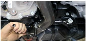
Tighten the clamp connecting the passenger muffler inlet pipe to the X-Pipe outlet using a ratchet and 15mm deep socket until muffler assembly is snug on the X-Pipe.
