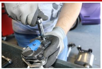
11. Line up the holes on the passenger actuator to the threaded spacers on the valve assembly. NOTE: There will be some resistance from the spring wire form as you rotated the actuator into position. This is normal as it applies pressure on the valve plate to the stops and prevents rattles.
