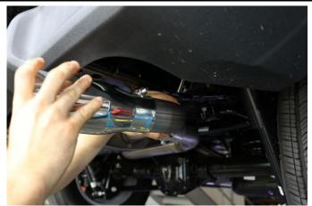
**8.** Slide the tips onto the tip elbow pipes with the etch centered on the top of each tip. Snug the bolt on the clamp using a 13mm socket or wrench.
