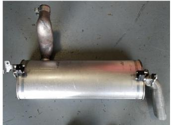
**3.** Remove the factory rear muffler from the vehicle by wiggling it back and forth while pulling. It may help to use a slight twist back and forth as well.
