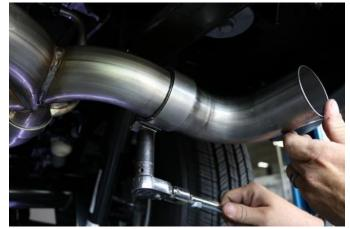
Place a clamp on the expanded end of the 90degree elbows with the hardware toward the front of the vehicle with the nut down. Then slide that end over the outlet pipe of the muffler. Use a 15mm socket or wrench to snug the clamp. Repeat for the other side.
