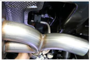
**3.** The use of a second person is recommended Slide the hangers into the factory grommets on both sides. Note: Use of a soap and water solution may aid in the installation of the hangers into the grommets.
