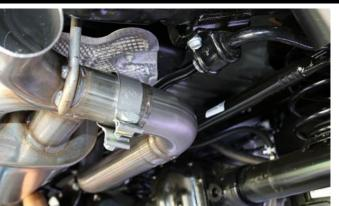
**4.** Slide the expanded inlet end of the rear muffler assembly onto the front section. Note: Make sure the clamp is on before you do this.
