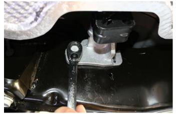
Re-install the driver and passenger hanger assemblies back in to their respective positions. Using the hangers/grommets from Removal Step 4 and the bolts from Removal Step 2.
