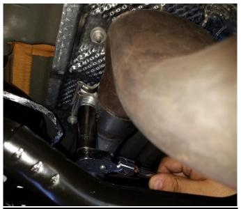
**1.** Loosen the factory clamp at the inlet end of the factory rear muffler assembly using a 15mm socket.
