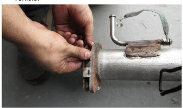
**9.** Remove the factory gasket from the muffler and save it to reuse for the Corsa system.
