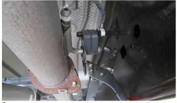
**4.** Remove hangers from the front of the muffler using grommet puller, or a similar device.
