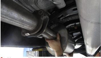
2. Line up muffler as shown in the picture. Align the flange to the mating flange of the mid pipe.
