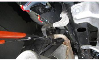
**6.** Remove hangers on the tailpipe using a grommet puller, or similar device.
