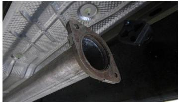
Place the gasket that was taken off from the factory exhaust system and place on the mid pipe flange.
