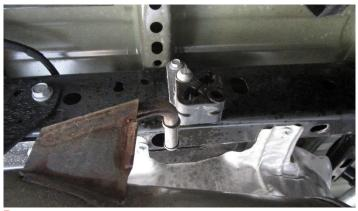
Carefully remove the passenger side tailpipe from the grommet and remove it from the vehicle.
