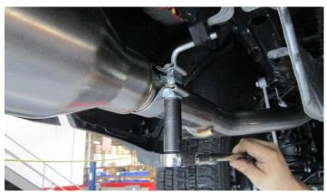
**12.** Using a 15mm socket or wrench, snug the tip clamps to leave room for adjustment.
