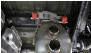
**3.** Place rear muffler hangers in the factory grommets.
