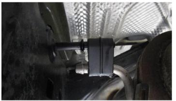
**4.** Place the front muffler hanger in the factory grommet.
