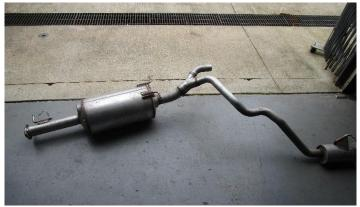
**8.** Carefully guide the rest of the system towards the front of the vehicle and down to remove the system completely of the vehicle.
