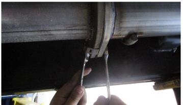
**5.** Using a 17mm socket or wrench and a 15mm socket or wrench, secure the flange connection with the supplied hardware.
