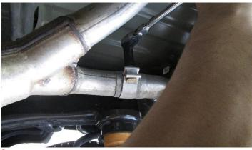
Loosen the passenger side tailpipe clamp using a 15mm socket or wrench.
