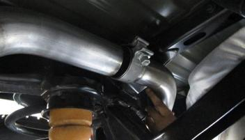
8. Install a 2.5" clamp into the inlet of the passenger rear tailpipe and insert the passenger rear tailpipe into the passenger front tailpipe. Place the passenger side rear tailpipe hanger into the factory grommet as shown in **Step 10.** Secure the clamp using a 15mm socket or wrench. Do not fully tighten at this time.
