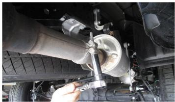
Loosen both of the tip clamps and remove the factory tip assemblies using a 13mm socket or wrench.
