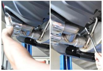
1. CAREFULLY insert the tip assembly into the driver side muffler outlet pipe and snug the clamp using a 15mm socket, 3/8" driver ratchet and 3" extension.
