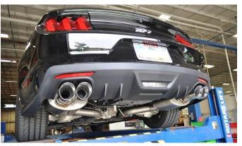
3. Adjust the position and depth of the tip assemblies until it is centered in the cutout, and has an equal amount of reveal on each side, then tighten the clamps using a 15mm socket and 3/8" ratchet. Torque the clamps to 45ft-lb using a torque wrench and 15mm socket, ensuring that the tips are still in the desired position.
