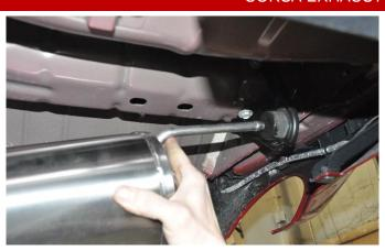
4. Slide the rear hanger into the rear hanger grommet located on the vehicle above and just inside of the passenger side tip cut out.
