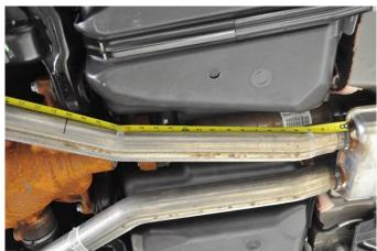
Measure 20" away from the flange on the stock resonator, following the outside profile of the exhaust pipe of the passenger side.
