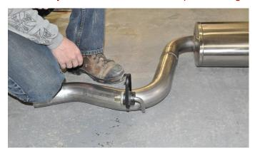
2. Locate the passenger side hanger grommet assembly removed during Removal Step 7 of the stock exhaust removal process along with the passenger side muffler assembly. Install the hanger grommet assembly onto the front hanger of the muffler assembly in the same position as previously installed on the stock exhaust.
