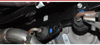
5. Once the bolt is removed, push up slightly on the exhaust and slide the hanger grommet assembly rearward to free it from the rear suspension subframe. Rotate the hanger grommet assembly a minimum of 90° so that it will not interfere with the rear suspension sub-frame.
