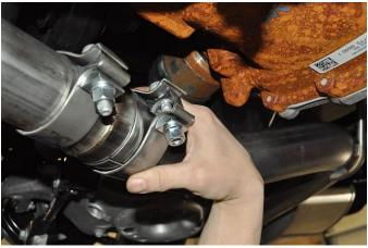
Slide the muffler inlet pipe over the passenger side adapter. NOTE: The use of a soap and water solution may aid in the installation of hanger grommets.
