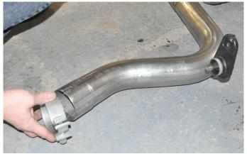
3. Locate one 3" clamp. Install the clamp on the passenger side muffler inlet pipe so that the bolt is vertical with the nut towards the ground and the bolt is towards the inside of the vehicle
