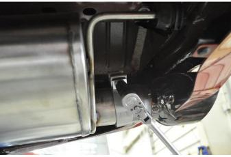
8. Locate the passenger rear tip assembly and one 3" clamp. Install the clamp on the tip inlet pipe so that the bolt is horizontal with the nut towards the inside of the vehicle and the bolt towards the top. Slide the tip assembly over the muffler outlet pipe and tighten the clamp using the ratchet and 15mm deep socket until the tip assembly is snug on the muffler outlet pipe. Repeat for the driver side tip assembly.
