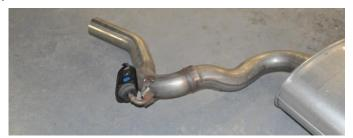
Remove both the driver and passenger side hanger grommet assemblies from the rear mufflers using grommet pullers or a similar device. Save the hanger grommet assemblies for reinstallation (Install Step 2).
