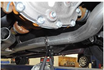
3. Using a chain cutter or similar device, cut both the driver and passenger side exhaust pipes at the marked locations. Place a jack stand or similar device under the stock tunnel section of the exhaust for support. Once the axle pipes are cut, there are no additional stock hangers supporting the tunnel section.
