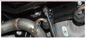
Using a 3/8" drive ratchet and 13mm socket, remove the **bolt** holding down the driver side hanger grommet assembly. Save bolt for reinstallation (Install Step 6).
