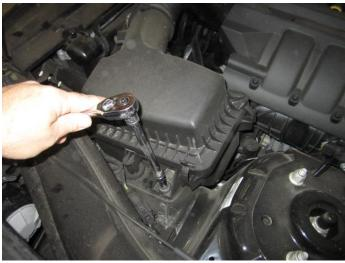
2. Remove the 10mm bolt holding the factory air box in place.
