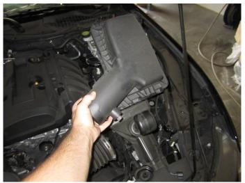
5. Remove the factory air box from the engine compartment.
