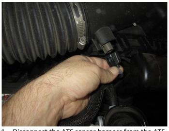
1. Disconnect the ATS sensor harness from the ATS sensor.
