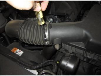
3. Remove the ATS sensor harness from the factory 4. Loosen the clamp holding the duct to the air box.
