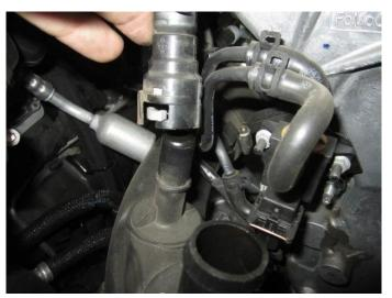
7. Remove the crankcase vent hose from the factory air duct.
