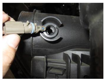
11. Remove the <u>ATS sensor</u> from the air duct. **Save for reinstallation**
