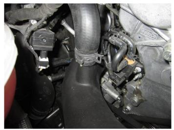
21. Attach the factory rubber hose to the CORSA duct using the factory clamp
