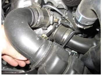
8. Loosen the clamp holding the factory air duct to the turbo.
