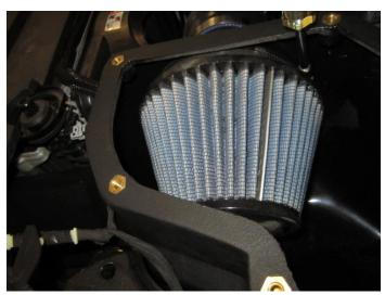
22. Attach the 5120 Ram filter onto the filter adapter using a 5/16 socket or nut driver only.
