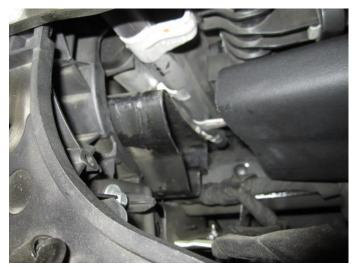
12. Slide the CORSA air box over the factory air inlet.
