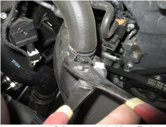
6. Using a pair of pliers remove the blow off valve hose from the factory intake duct.
