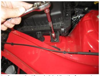
1. Remove the 10mm bolt holding the factory air box in place.
