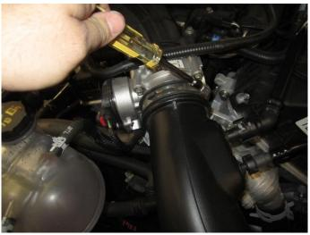
3. Loosen the clamp holding the duct to the throttle 4. Disconnect the factory breather hoses from the body.
