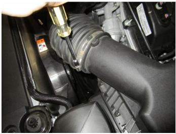
2. Loosen the clamp holding the duct to the air box.
