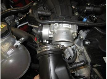
5. Remove the duct from the throttle body.
