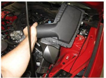
7. Remove the factory air box from the engine compartment.
