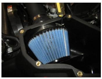
18. Tighten the #5120 Pro-5 filter onto the adapter using a 5/16 socket or nut driver only.
