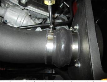
14. Tighten the clamp holding the duct to the hump hose using a 5/16 socket or nut driver only.
