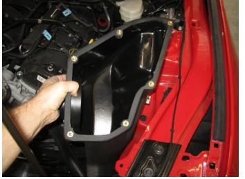
Place the CORSA air box into the factory location the air box will slide over the factory inlet.
