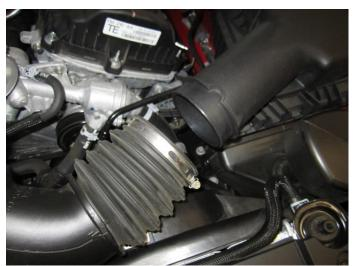
6. Remove the duct from the air box then remove the air duct from the engine compartment.
