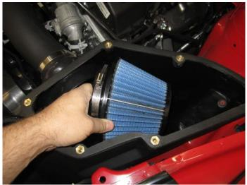
17. Slide the #5120 Pro5 filter onto the filter adapter.
