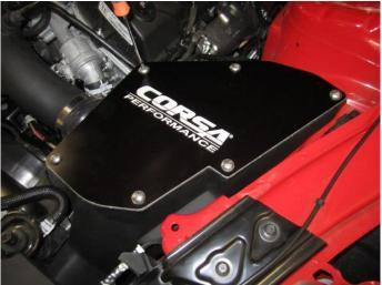
19. Attach the CORSA air box lid using the provided truss head screws and rubber washers. Check all connections and clamps before starting the vehicle. Reattach the negative battery cable and retighten all connections after 100, 500 and 1000 miles. Reconnect the battery cable.
