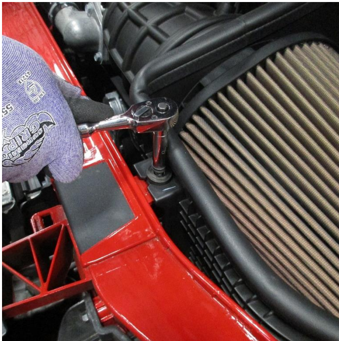
7. Remove the bolt securing the factory air box. The bolt will be reused during installation.
