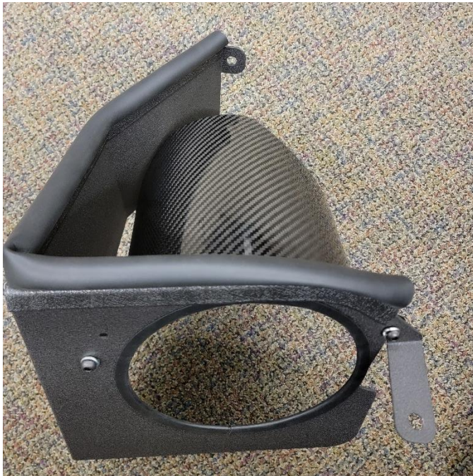
3. Install CORSA Carbon Fiber rain guard onto heat shield with M6x12mm bolts, flat washers and M6 nuts.
