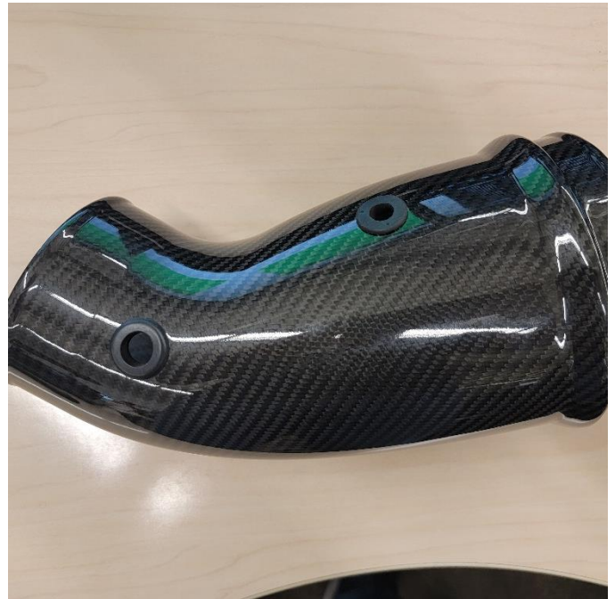
4. Install \text{Ø}5/8 " ID grommet into CORSA Carbon Fiber air duct in hole closest to small end. Install \text{Ø}1/2 " ID grommet into CORSA Carbon Fiber air duct in hole closest to large end.
