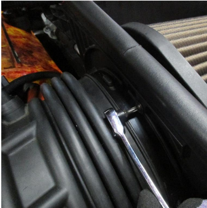
5. Remove the bolts securing the air filter to the factory air box.
