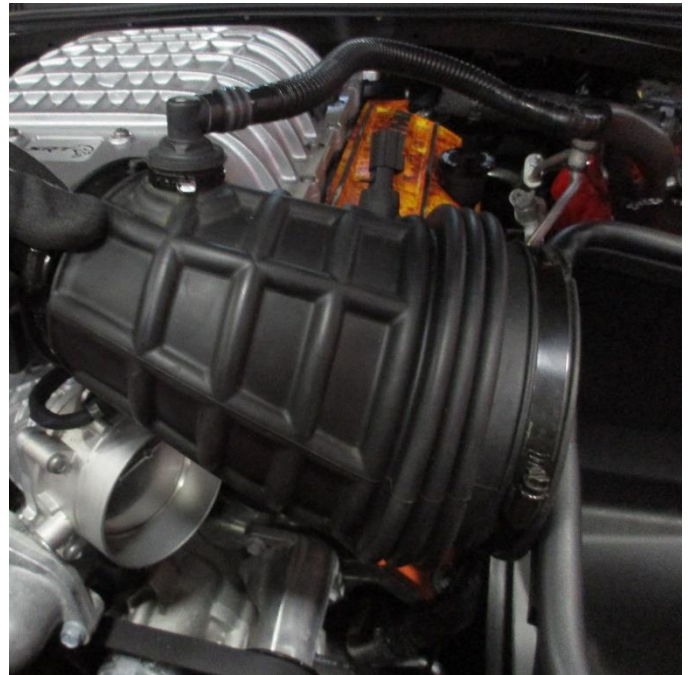
10. Remove the factory air duct assembly along with the vent hose and solenoid from the vehicle.
