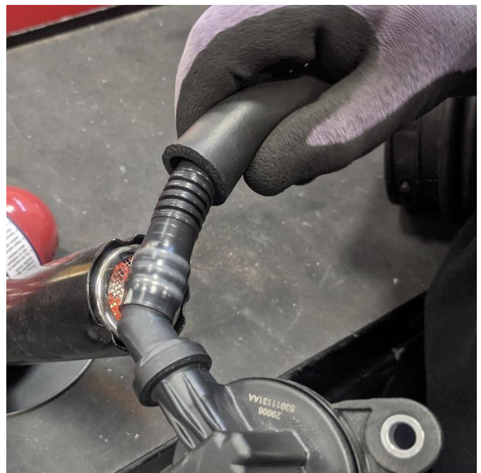
12. Use a heat gun to warm the factory vent hose at the connection to the solenoid. Disconnect the hose from the solenoid.
