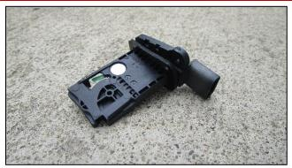
Install CORSA MAF gasket onto MAF sensor.
