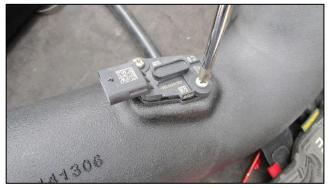
Install sensor into CORSA air duct. Secure using the two supplied screws and a Philips head screwdriver.
