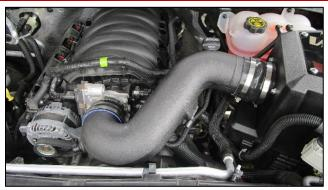
Insert CORSA air duct into hump hose and straight sleeve.
