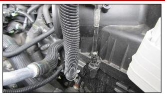
Remove three bolts securing factory air box upper portion to lower using a ratchet with extension and 8mm socket.
