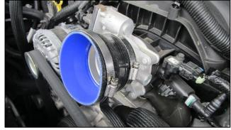
**6.** Place straight sleeve onto throttle body with included #64 clamp. Place included #64 clamp on other end of straight sleeve.
