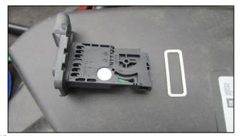
12. Remove factory gasket from MAF sensor.
