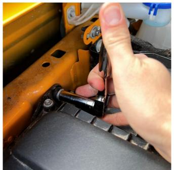
Use a 10mm socket and rachet to remove the bolt located behind the stock air box. Save bolt for installation step 12.
