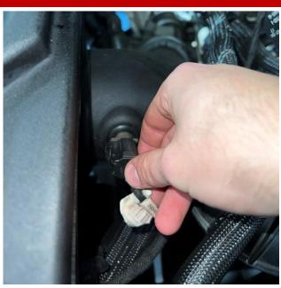
Re-attach electrical connection to the temperature sensor by pressing until it clicks into place.
