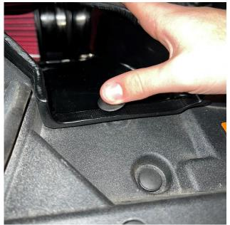
**12.** Use the supplied Christmas Tree clip to secure the scoop portion of the CORSA airbox to the stock air intake tray.
