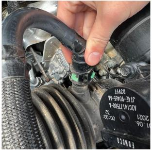
Remove the PCV line by pressing the green tabs on the fitting up and out then pulling the fitting off.
