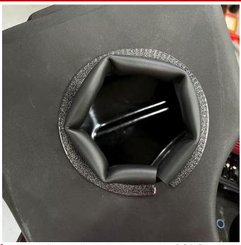
Install filter bulb seal trim onto the CORSA air box.
