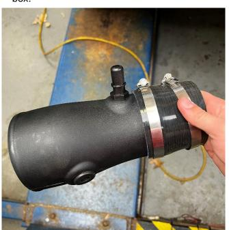
3. Install the silicone reducer to the smaller end of the CORSA air duct. Prep the Ø3.5" and Ø3.25" clamps for install by sliding them over the silicone reducer. Use an 8mm socket and ratchet to tighten the Ø3.5" clamp over the duct. Leave the Ø3.25" clamp loose for installation.
