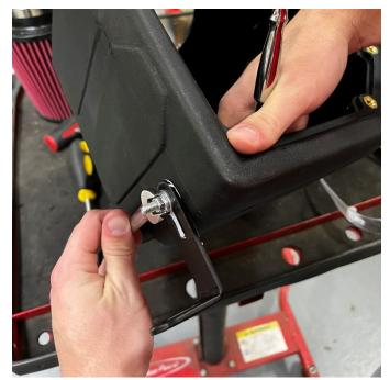
8. Install the bracket to the drilled hole on the back of the CORSA air box using the supplied bolt, nut, and washer. Use a 10mm socket ratchet and wrench to tighten.
