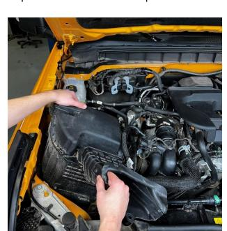
Carefully remove the stock air intake by pulling up and out.
