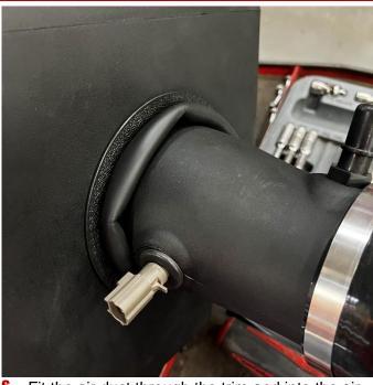
Fit the air duct through the trim and into the air box.
