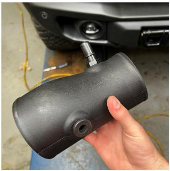
Install the rubber grommet and thread the fitting onto the CORSA air duct.
