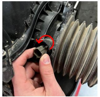
**8.** Carefully remove the temperature sensor from the stock air intake by rotating counterclockwise and pulling out. Save temperature sensor for installation step 4.
