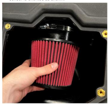
Install the air filter and air filter clamp directly over the end of the air duct inside the air box. Use an 8mm Socket to tighten. Fit pre-filter over top of filter if desired.
