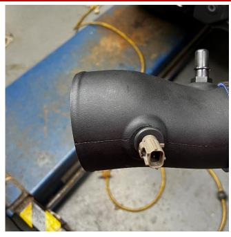
**5.** Install the temperature sensor to the air duct by fitting it through the rubber grommet. Make sure sensor is oriented as shown.
