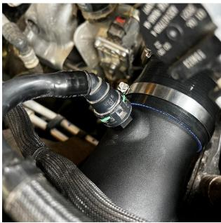
9. Carefully install CORSA air intake and fit the silicone reducer over the stock turbo inlet pipe. Tighten Ø3.25" clamp reconnect the PCV line to the Volant air duct by pressing it over the fitting until it clicks into place.
