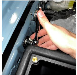
11. Align the supplied bracket to the threaded hole in the frame and use a 10mm socket and the stock bolt from removal step 3 to secure the CORSA airbox to the vehicle.
