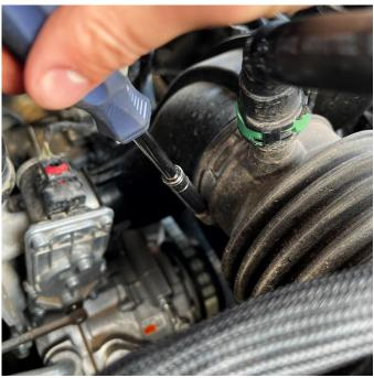
Loosen the clamp securing the air duct to stock turbo inlet pipe using and pull the duct off the inlet pipe.
