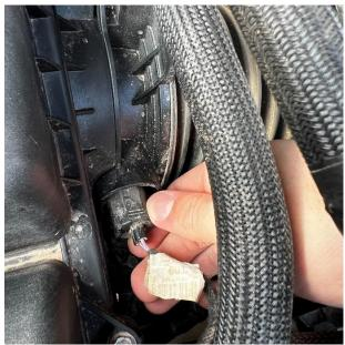
Disconnect the electrical connection on the air temperature sensor by pressing on the tab and pulling.
